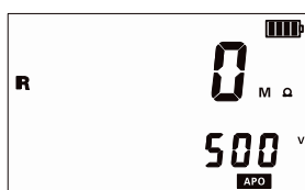
Figure 9-4 Insulation resistance measurement mode
