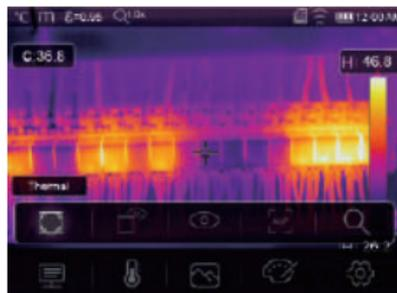
Thermal Imager has 5 kinds of image modes for display: Thermal, Picture in Picture, Camera, Auto Fusion, Measuring Distance.
