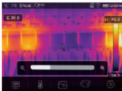
In the Zoom mode, press the left key or slide the zoom bar to zoom in the image. Press right Key or slide the zoom bar zoom out the image.
