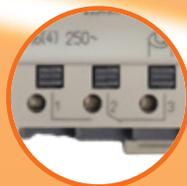
Normally Open & Normally Closed Switching Terminals
