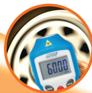
Measuring speed of a rotating object
