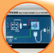
3.5" TFT Colour LCD Display with 320x240 Pixels
